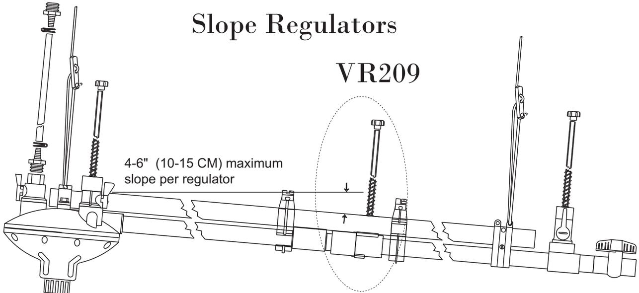
NOTE: Be sure to place the hanger bracket flush against the regulator, to prevent tipping.
