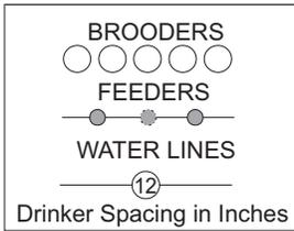
**NOTE:** In 1/2 or 1/3 house brooding, water lines may be sectioned off or continuous up to 400 FT (122 M) in length. Contact VAL-CO Watering Systems for technical advice on sloped houses or other floor plans desired.
