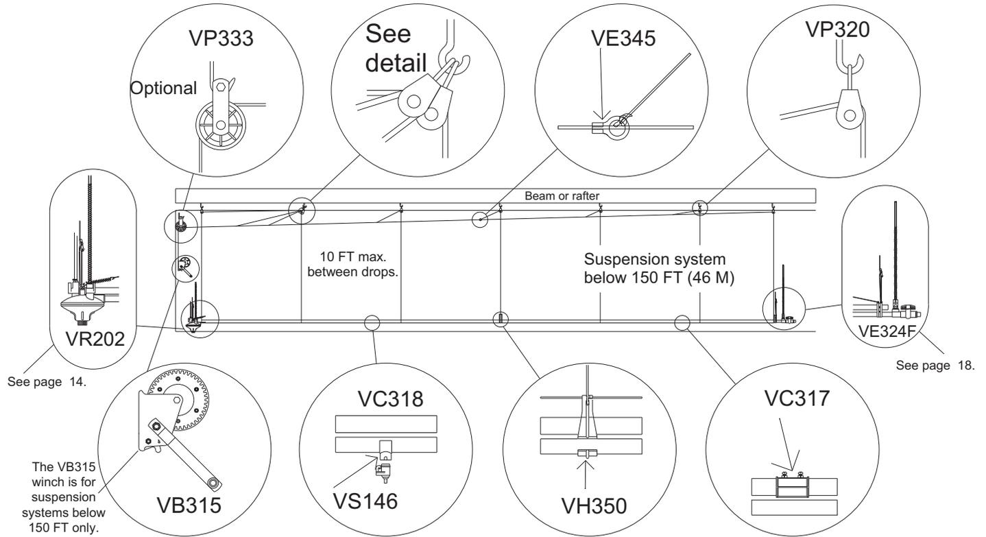
Split winch (VB312) should be used for suspension systems 150 FT (46 M) and over.
