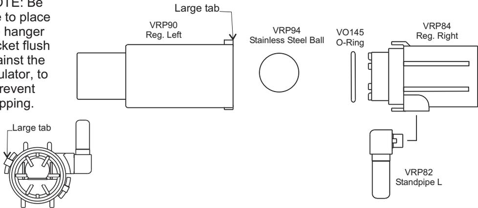
Slope regulators should be used when the column height at the end assembly is 6" (15 CM) or higher than the column height at the supply regulator (VR202).
