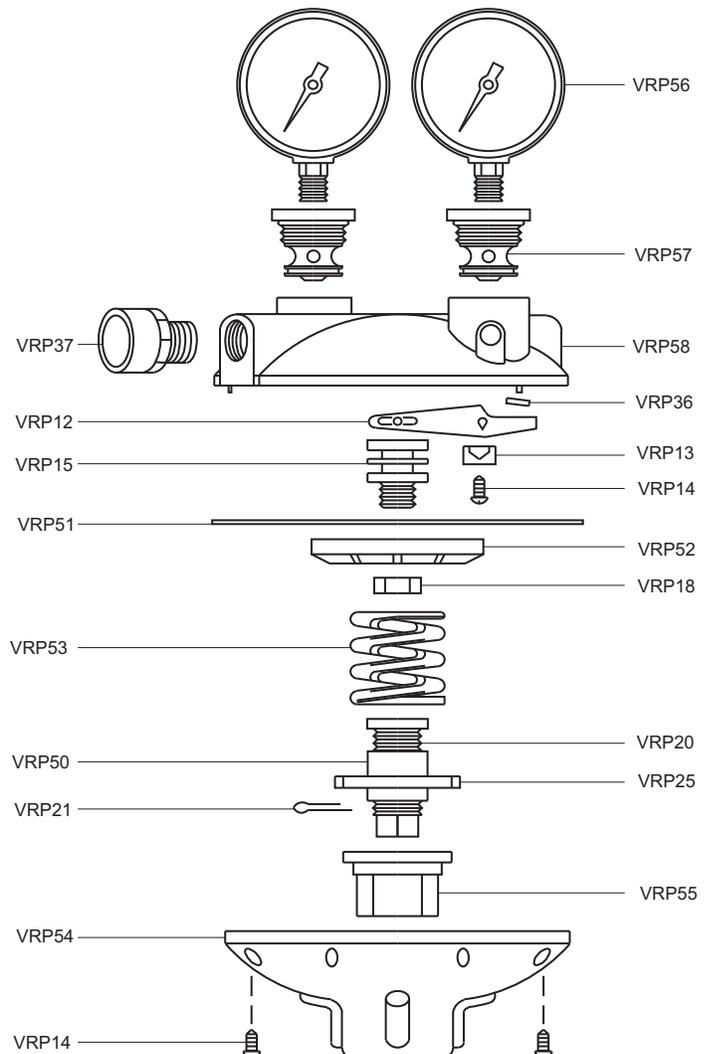
The high pressure regulator should be used when incoming water fluctuates more than 20 PSI (1.7 Bar). Set the outlet pressure at least as low as the lowest pump pressure setting, which will maintain an even outlet pressure. Do not set regulator pressure below 25 PSI.
