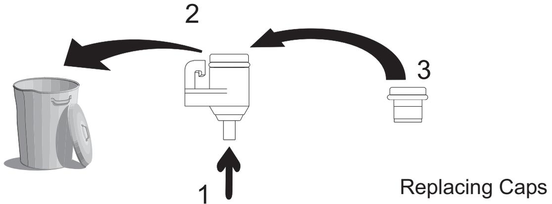
1. Push up on the stainless steel pin to loosen the old plug.
