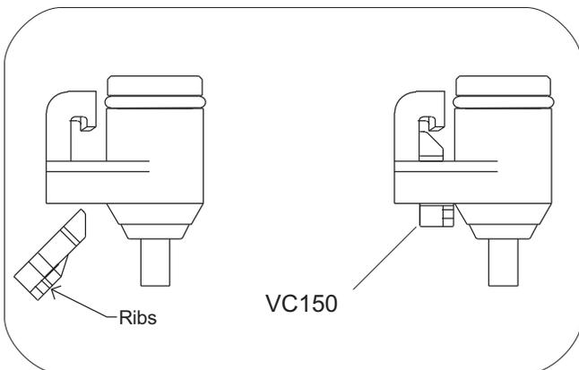
The ribs on the clip should face the nipple body.
